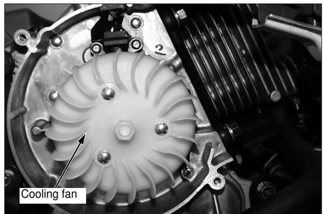
Remove the A.C generator flange nut.
